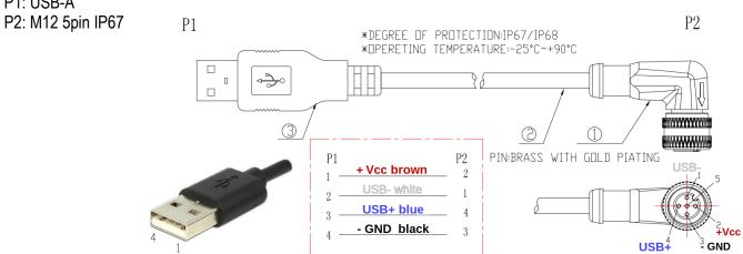
For industrial and building automation a star topology on 24VDC power supply is recommended using the M12 ready made power supply cables. For data offloading a M12 to USB cable can be used.
