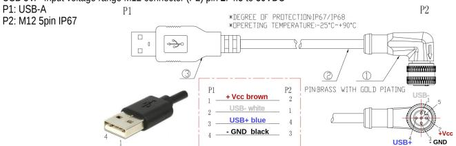
For industrial and building automation a star topology using T-cable-splitters of 24VDC power supply is recommended. The standard M12 cables have molded IP67 connectors on both sides (Male, Female)
