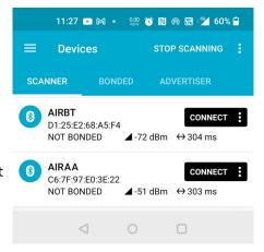
The app also shows the bluetooth signal strength. In the example -51 dBm for the anchor and a weaker signal of -72dBm for the tag 'AIRTBT' mainly because of a larger distance between the phone and device. The signal strength gets weaker when the phone is a few meters away from the device compared to close by. The phone can be 10+ meter away and still update the device. In case of packet loss the process takes longer.
